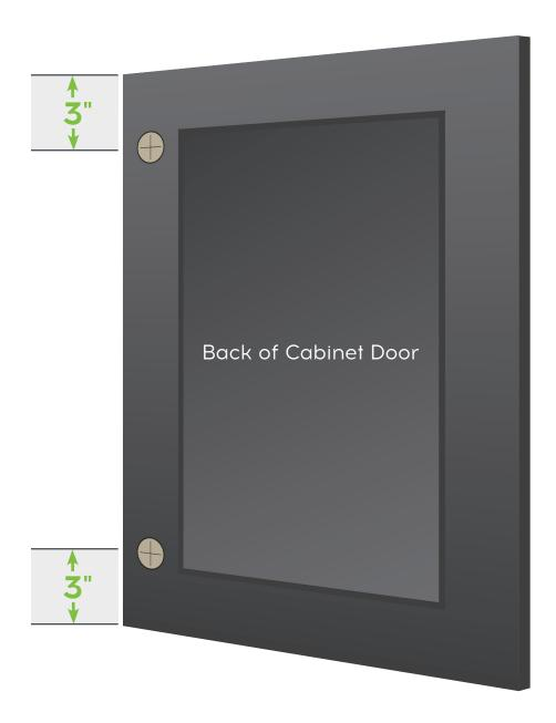
Measure the distance from the bottom & top of the cabinet to the MIDDLE of the bore hole.
