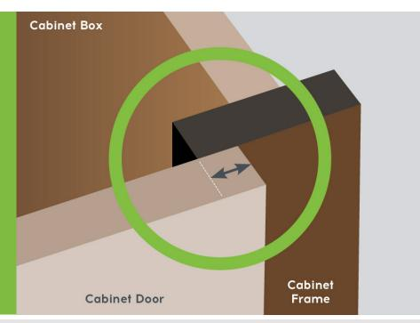
How to Calculate Hinge Overlay (Step by Step)
